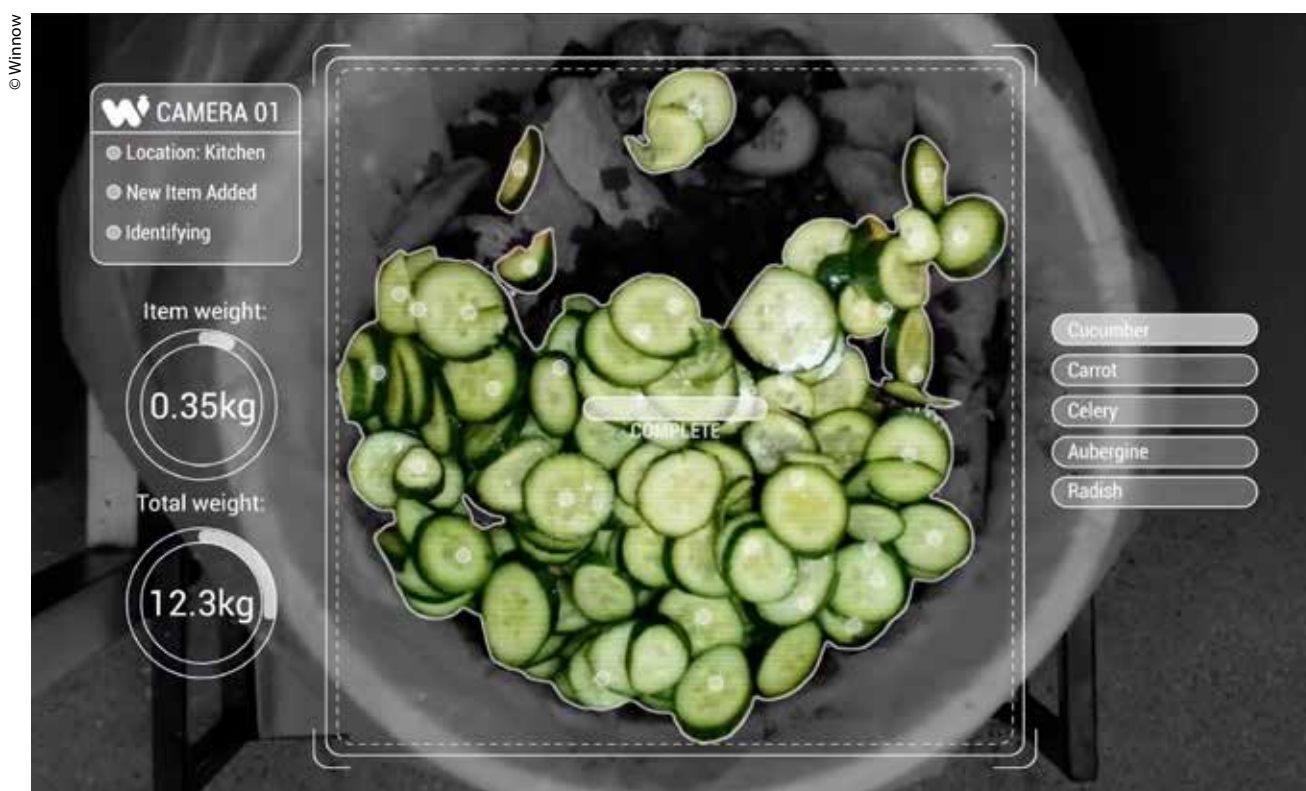
▼ Winnow, an AI tool developed in the UK, analyzes food waste using a camera installed above a bin.
